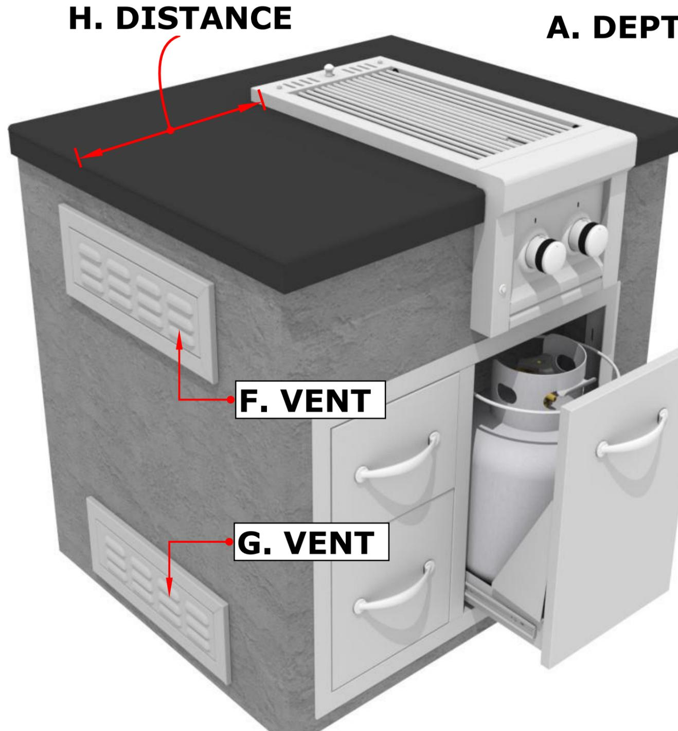
CUT-OUTS ARE GIVEN 1,91cm MINIMUM AIR FLOW VENT BELOW THE GRILL DRIP PAN.
